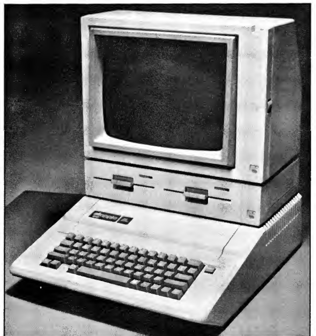
Duodisk contains two half-high drives side-by-side.
